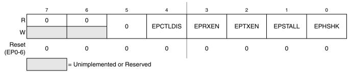
Figure 17-17. Endpoint Control Register (EPCTLn)
