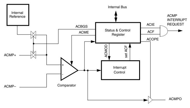
Figure 9-2. Analog Comparator 5V (ACMP5) Block Diagram
