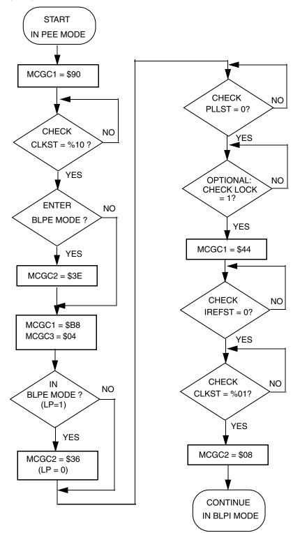
Figure 12-10. Flowchart of PEE to BLPI Mode Transition using a 4 MHz Crystal
