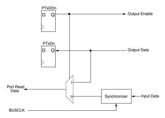
Figure 6-1. Parallel I/O Block Diagram
