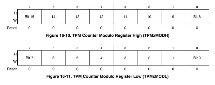
Reset the TPM counter before writing to the TPM modulo registers to avoid confusion about when the first counter overflow will occur.
