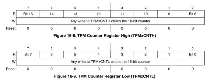
When BDM is active, the timer counter is frozen (this is the value that will be read by user); the coherency mechanism is frozen such that the buffer latches remain in the state they were in when the BDM became active, even if one or both counter halves are read while BDM is active. This assures that if the user was in the middle of reading a 16-bit register when BDM became active, it will read the appropriate value from the other half of the 16-bit value after returning to normal execution.
