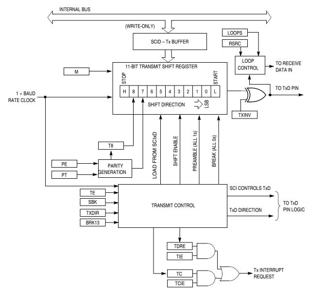
Figure 14-2. SCI Transmitter Block Diagram
