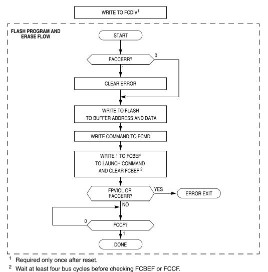
Figure 4-2. Flash Program and Erase Flowchart
