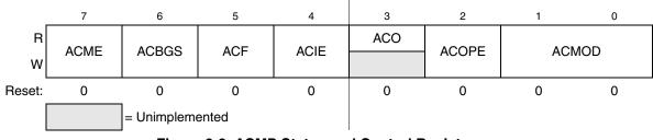
Figure 9-3. ACMP Status and Control Register
