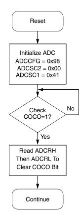
Figure 10-13. Initialization Flowchart for Example
