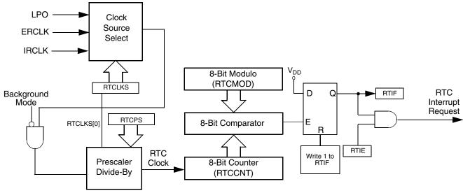
Figure 13-2. Real-Time Counter (RTC) Block Diagram
