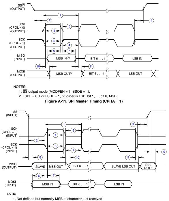
Figure A-12. SPI Slave Timing (CPHA = 0)
