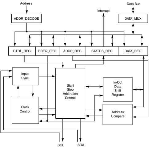
Figure 11-2. IIC Functional Block Diagram
