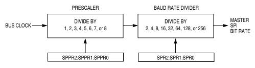
Figure 15-15. SPI Baud Rate Generation
