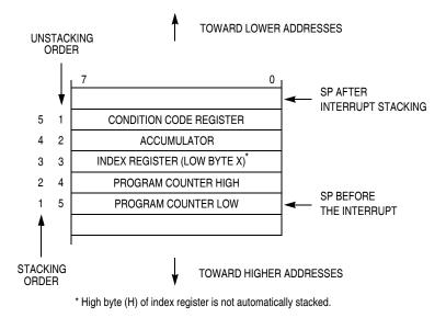
Figure 5-1. Interrupt Stack Frame
