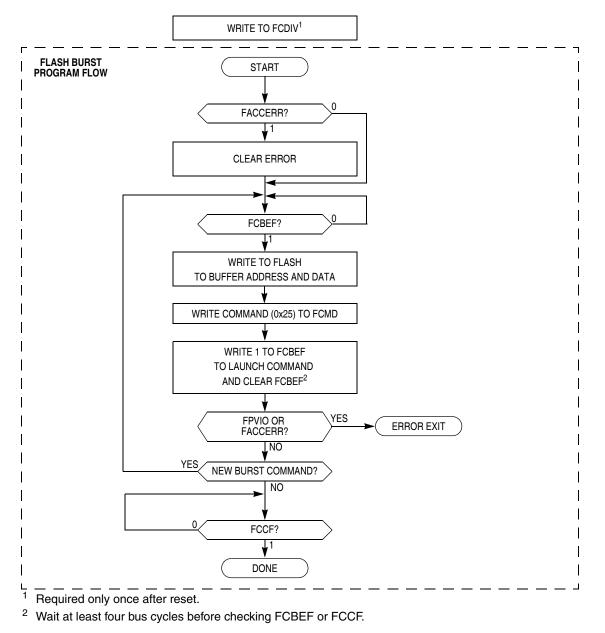
Figure 4-3. Flash Burst Program Flowchart
