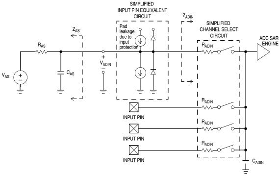
Figure A-5. ADC Input Impedance Equivalency Diagram
