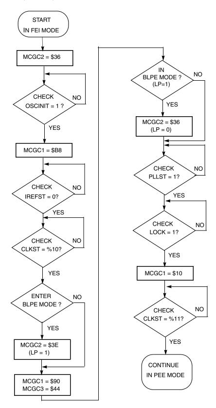
Figure 12-9. Flowchart of FEI to PEE Mode Transition using a 4 MHz Crystal
