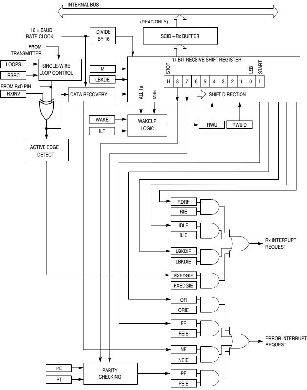
Figure 14-3. SCI Receiver Block Diagram
