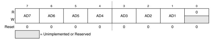
Figure 11-3. IIC Address Register (IICA)
