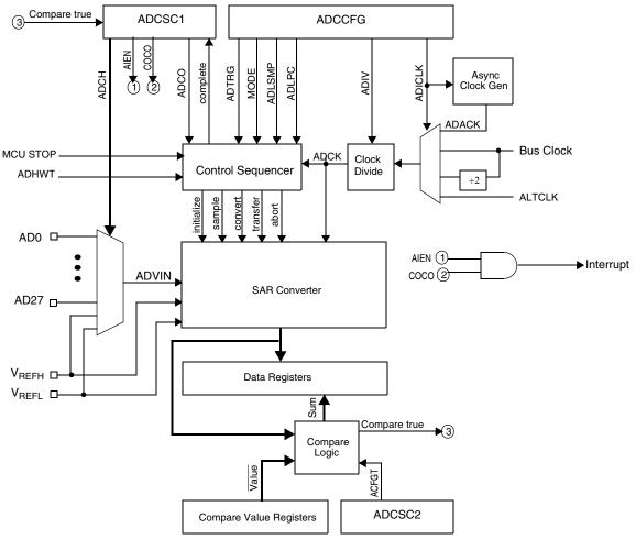
Figure 10-2. ADC Block Diagram
