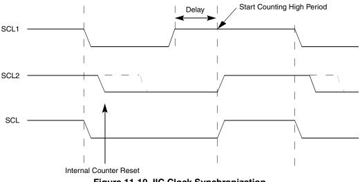
Figure 11-10. IIC Clock Synchronization
