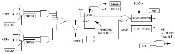
Figure 8-2. KBI Block Diagram
