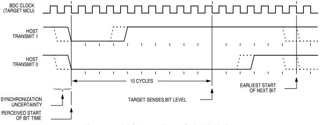
Figure 18-2. BDC Host-to-Target Serial Bit Timing
