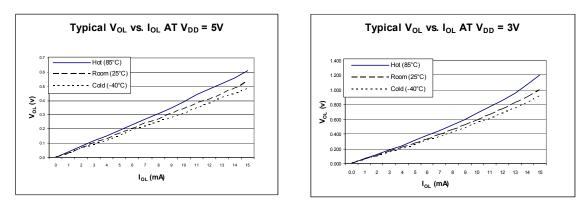
Figure A-1. Typical Low-Side Drive (Sink) Characteristics – High Drive (PTxDSn = 1)
