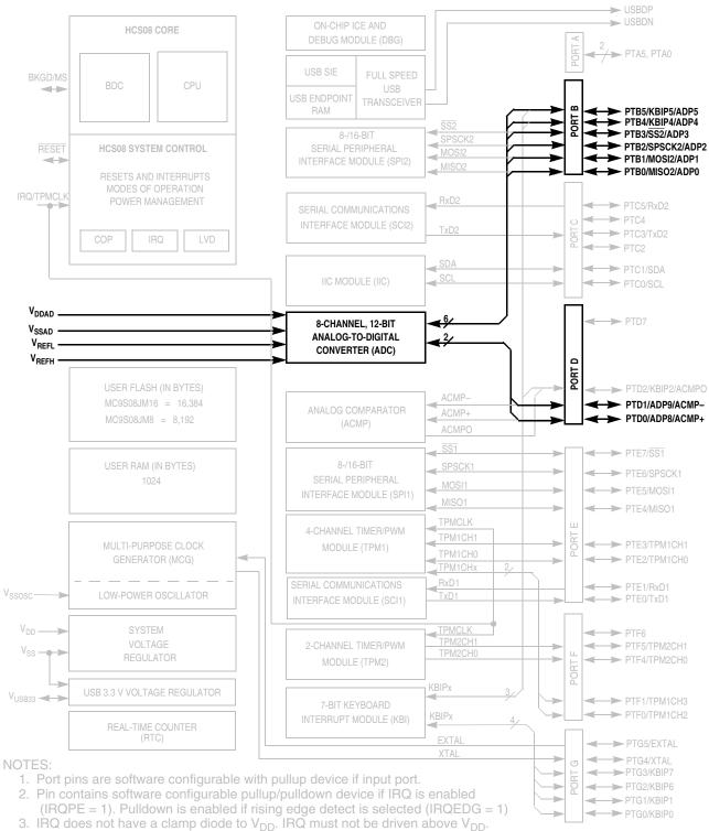
4. Pin contains integrated pullup device.
