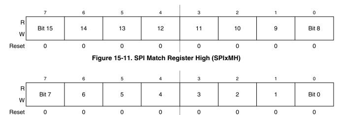
Figure 15-12. SPI Match Register Low (SPIxML)
