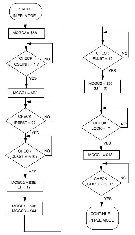
Figure 12-12. Flowchart of FEI to PEE Mode Transition using a 8 MHz Crystal
