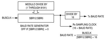
Figure 14-12. SCI Baud Rate Generation
