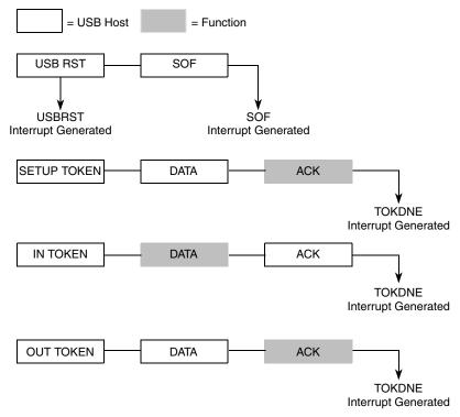
Figure 17-20. USB Packet Flow
