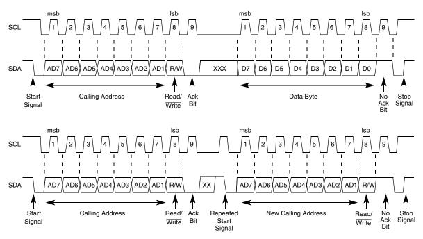
Figure 11-9. IIC Bus Transmission Signals
