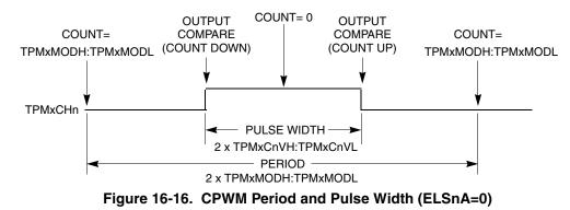
Center-aligned PWM outputs typically produce less noise than edge-aligned PWMs because fewer I/O pin transitions are lined up at the same system clock edge. This type of PWM is also required for some types of motor drives.
