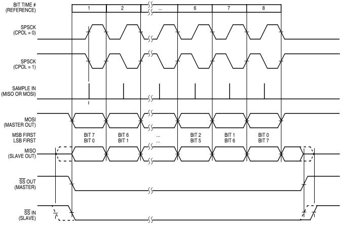
Figure 15-14. SPI Clock Formats (CPHA = 0)
