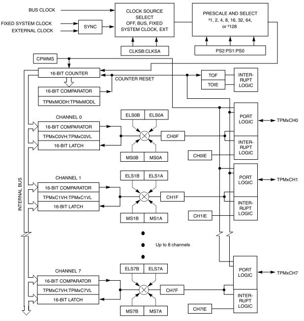
Figure 16-2. TPM Block Diagram
